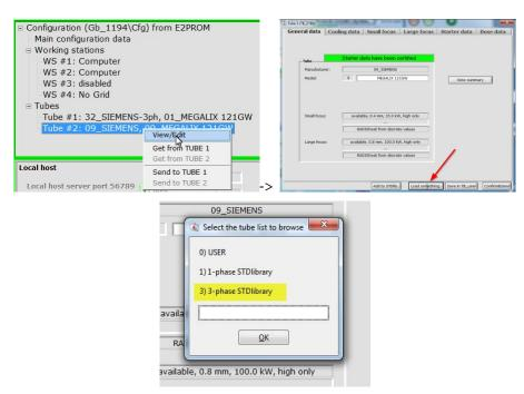
Opening up the possibility of selecting tubes with three-phase stators.
